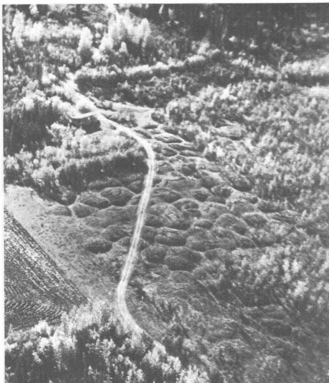
FIGURE 10.—Thermokarst mounds near Fairbanks. Mounds range from 10 to 30 feet in diameter. See figure 11 for ground view of mounds and explanation. Photograph by R. F. Black and T. L. Péwé, September 1948.
