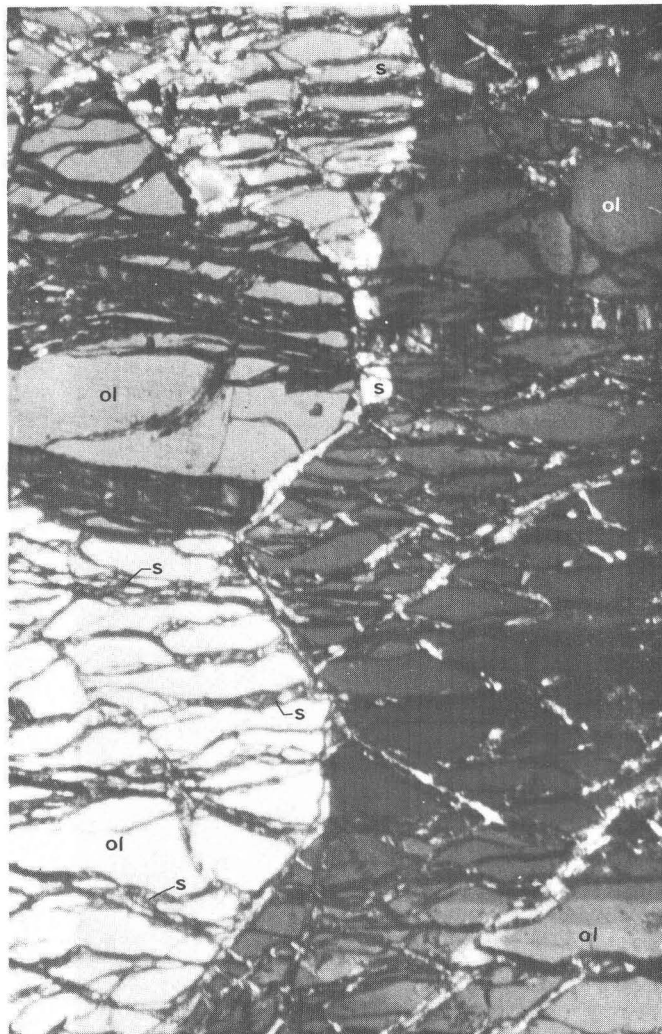
Figure 3.—Strongly sheared and serpentinized dunite. Serpentine veinlets form complex anastomosing network. ol, olivine; s, serpentine.
