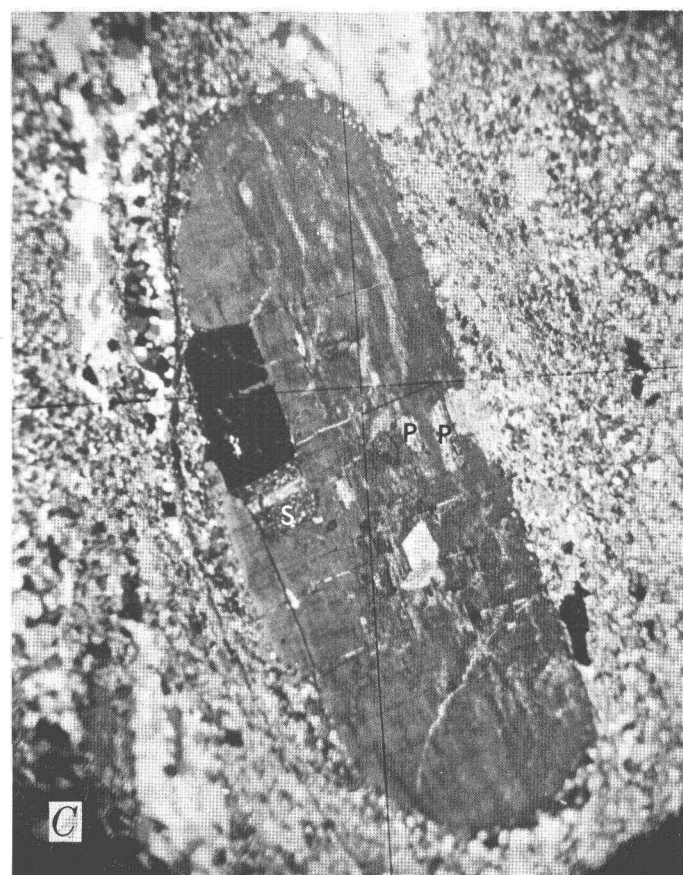
FIGURE 10.—Perthitic microcline megacrysts in granite. Crossed polars. A, Euhedral crystal showing marginal growth (M) into fine-grained groundmass. Okpilak River, east fork. B, Euhedral crystal with rounded corners possibly the result of granulation. Arey Creek. C, Ovoidal megacryst showing marginal growth into fine groundmass. Optically oriented plagioclase (P) within crystal. Small square area (S) is sericitized plagioclase not oriented with long axis of megacryst. Creek four miles south of Okpilak Lake. All photos at same scale.
