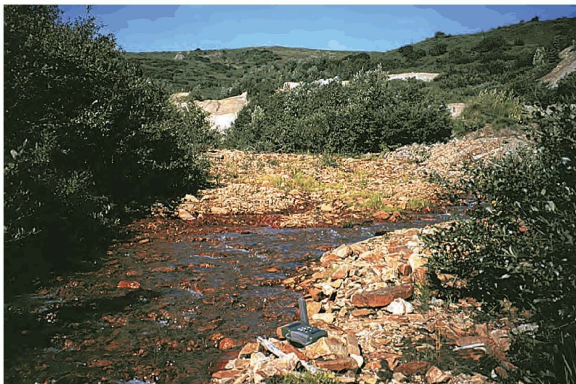
Figure 5. Site 98SC007 (pH value, 6.9; conductivity, 260 \mu\text{S}/\text{cm} ; total-dissolved-solids content, 246 mg/L) on Slate Creek immediately below the Slate Creek antimony deposit (see figs. 1, 3 for location). Red Fe oxide coatings on alluvial cobbles are common along much of lower Slate Creek. Mine wastepiles are visible in distance; Global Positioning System (GPS) unit in foreground for scale.
